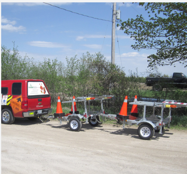
Two trailers can be towed in tandem due to extra hitch.
