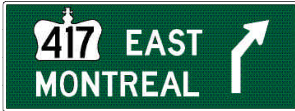
Figure 2.13 CHANNELIZING – RIGHT TURN Sign (Gr-1)
