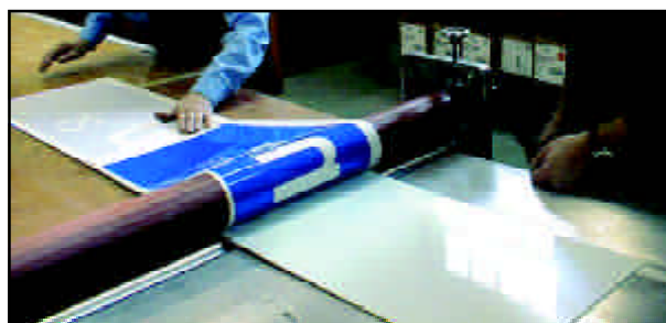
Figure 4.27 – Application of Transfer Tape and Reverse-cut Transparent Sheeting to Reflective White Background Sheeting on Substrate
