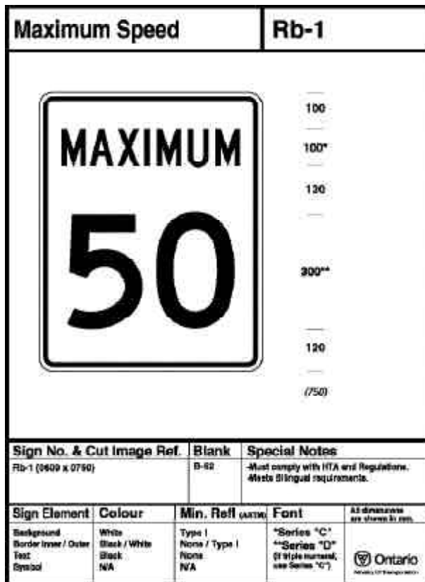
Figure 5.1 – Sign Pattern Template for Rb-1
