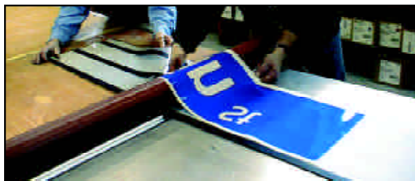
Figure 4.25 – Stripping of Backing from Reverse-cut Transparent Sheeting (first half)
